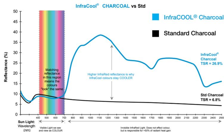
This chart shows the "Spectral Reflectance" of InfraCOOL® Charcoal vs Standard Charcoal. Its the way we measure reflectance of sun light across the full spectrum. The rainbow portion depicts the wave lengths of light in the "visible spectrum" which determines colour as we see it.
